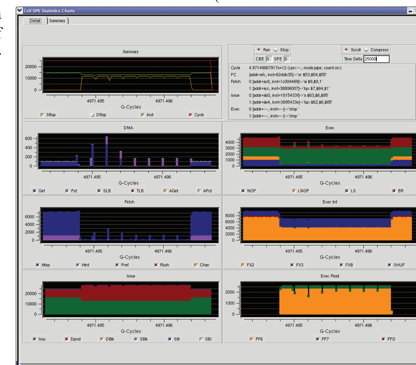
(2) Screenshot of performance data generated using the Cell Simulator provided by IBM. This figure is a single iteration of a 2D stencil program written using Charm++ and the Offload API. This run utilizes all 8 SPEs on the Cell. Each SPE receives 8 evenly sized chunks of data.
