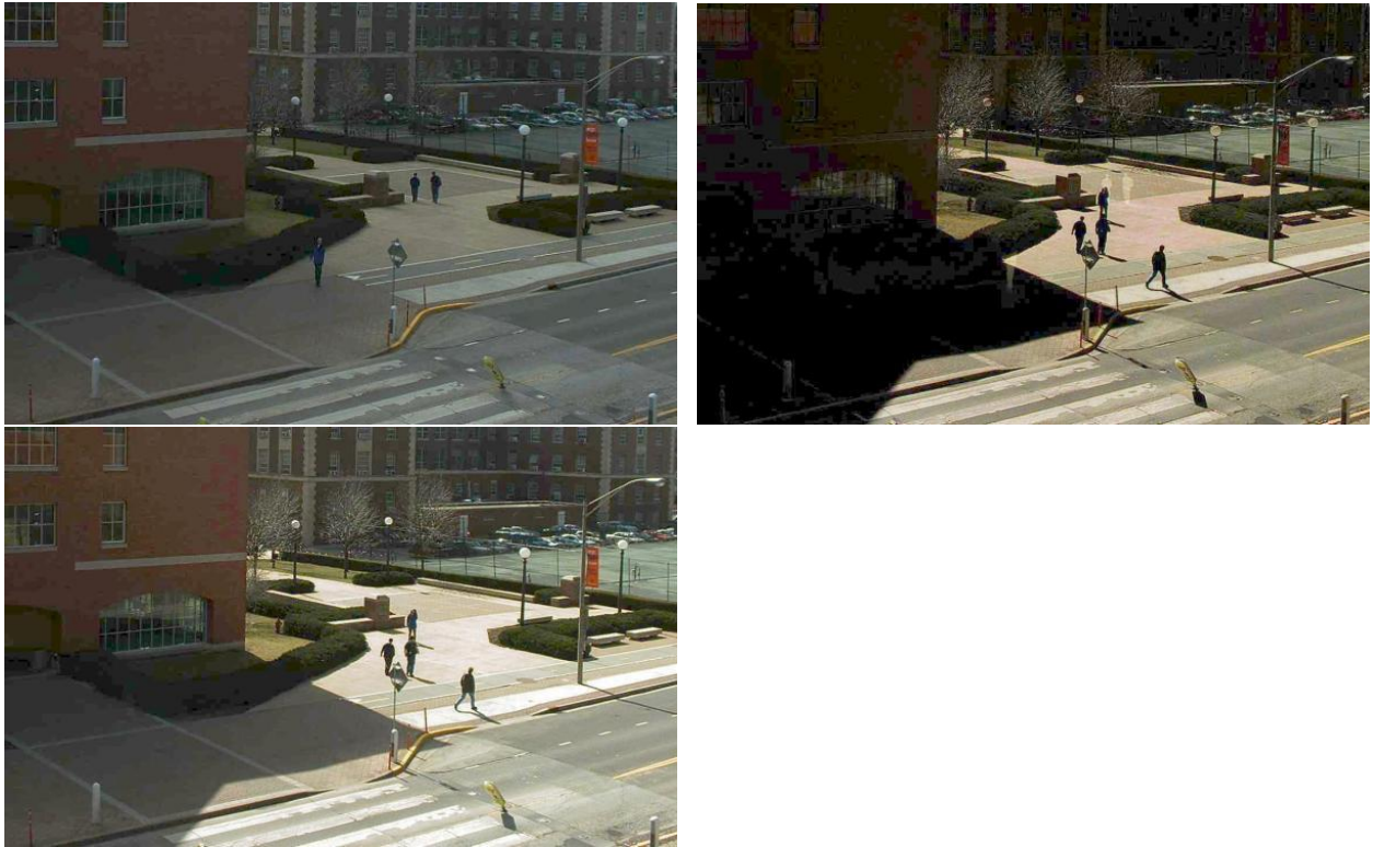
Figure 6.3. Campus illuminated by sky light (top), sun light only (middle), and sun and sky light (bottom). The top and bottom images are calibrated photographs acquired with a digital camera; the sun-only image is computed from these images by subtracting the sky light image from the sun and sky light image.
