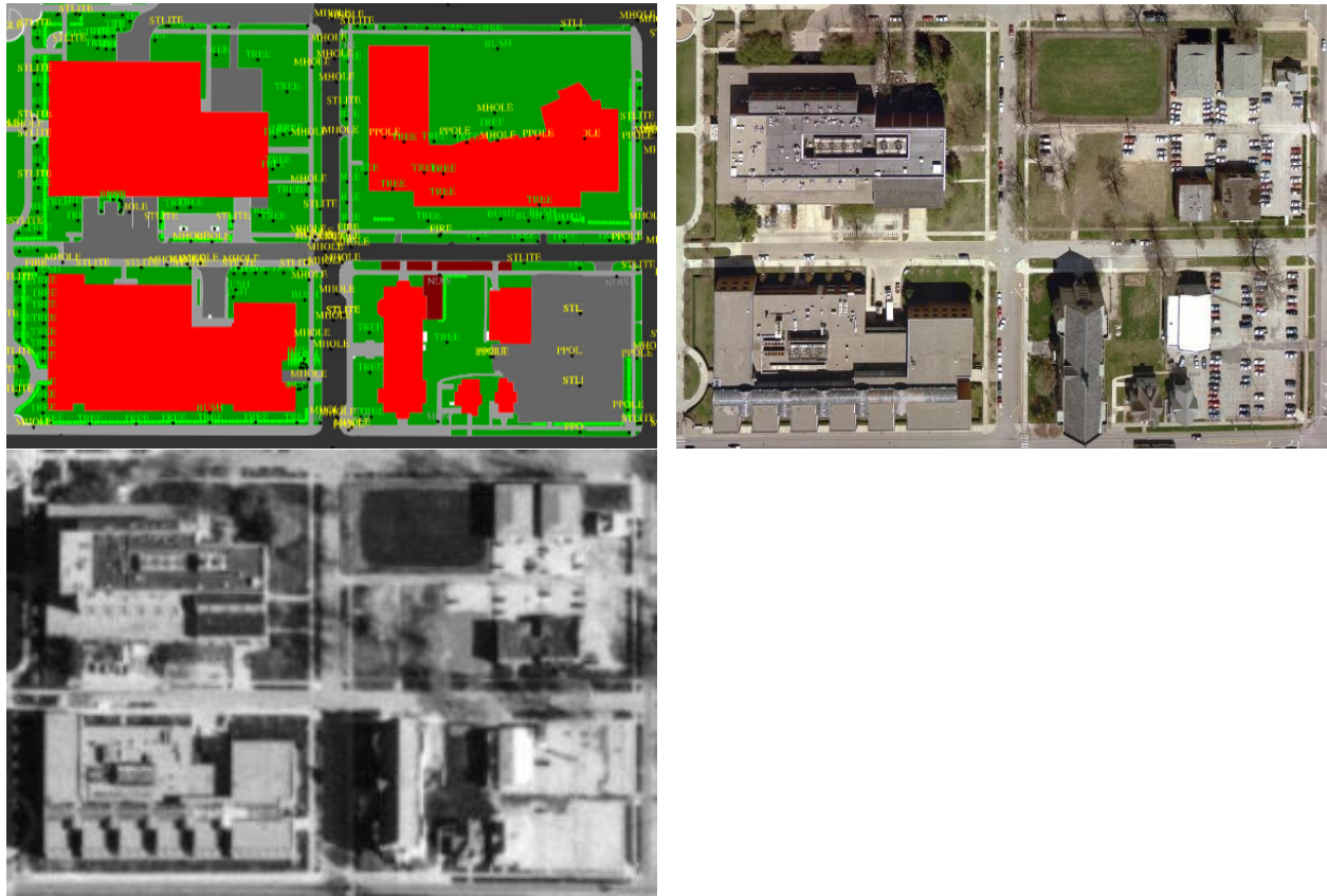
Figure 7.10. Four blocks from the 2004 campus utilities map (top) and 1999 aerial photo (middle), and 1998 USGS orthophoto (bottom) near Goodwin and Springfield Avenue in Urbana, Illinois. Note how the Siebel Center in the top right, constructed in 2003, does not appear in the lower two photos.
