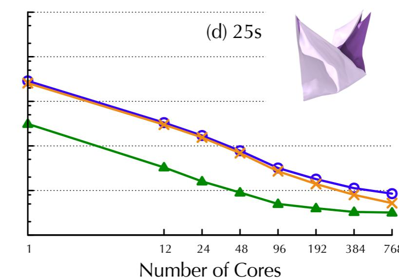
Time per window —○— Force calculation —×— Collision detection —▲—
