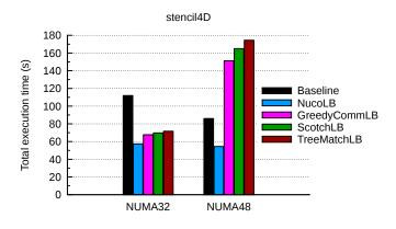
Fig. 4. Comparison of different load balancers for the stencil4D benchmark.
