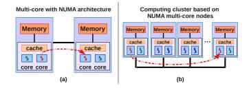
Fig. 1. Communication on hierarchical parallel machines.
