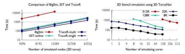
**Figure 4:** Comparison of the sequential execution time of TraceR with that of BigSim and SST for 3D tori of different sizes (left). Weak and strong scaling performance of TraceR simulating 3D tori of different sizes on different core counts (right).
